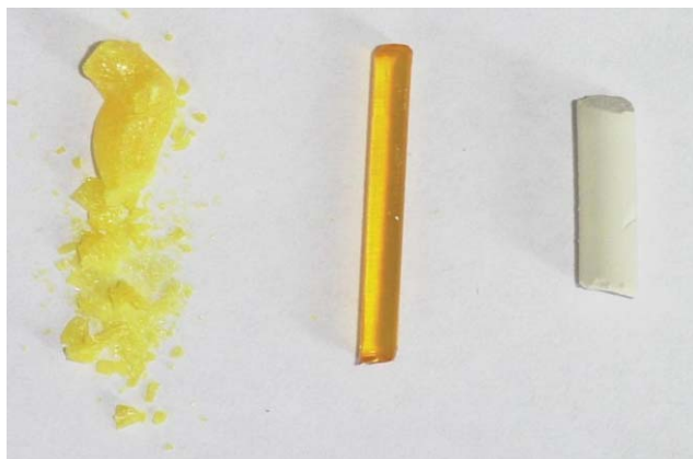
Fig. 1 Xerogel powder (left), xerogel monolith (center; 2.5 mm diameter), and aerogel monolith (right; 4.1 mm diameter) prepared from 2 . In the wet gel stage, the samples had about the same diameter as that of the aerogel sample, i.e. the xerogel monolith shrank to about 60% of its original size during drying.
